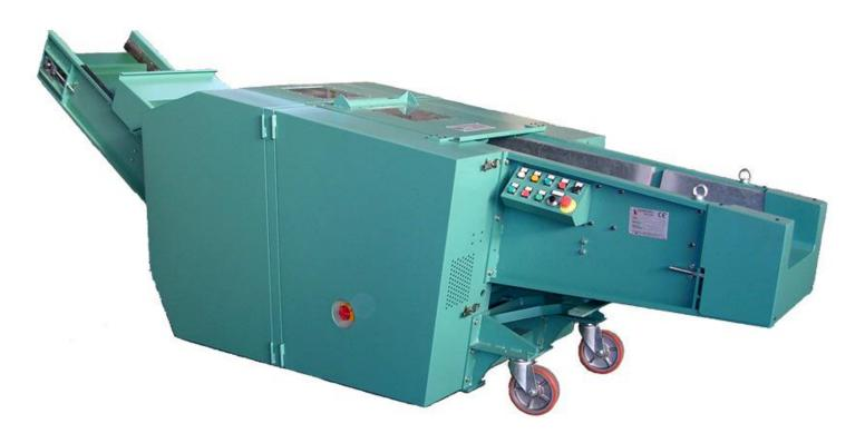
The rotating blades are helicoidally shaped which ensures a perfect cut on the entire 500 mm width and also distributes the cutting load over the length of the blades.
