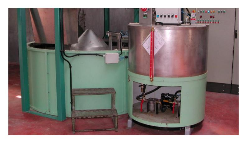
New studies and experiments carried out in view of the various problems connected with the application of oil and other additives have led to the realisation of the **new spraying system for direct application to the fibres being fed into the blending bins via conveyor belts**.
