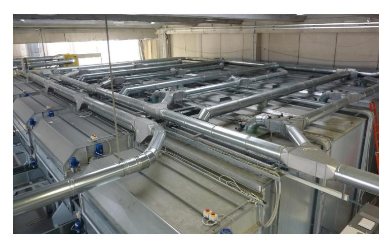
Setting system is very performing and allows to feed an extrusion line with more than **2.000 Kg/h** of regenerate products. Is handled automatically leaving to the operator the task to put the raw material on the conveyor stacker, from where the cycle do not need any manual intervention up to the storage of pallets of finished cips.
