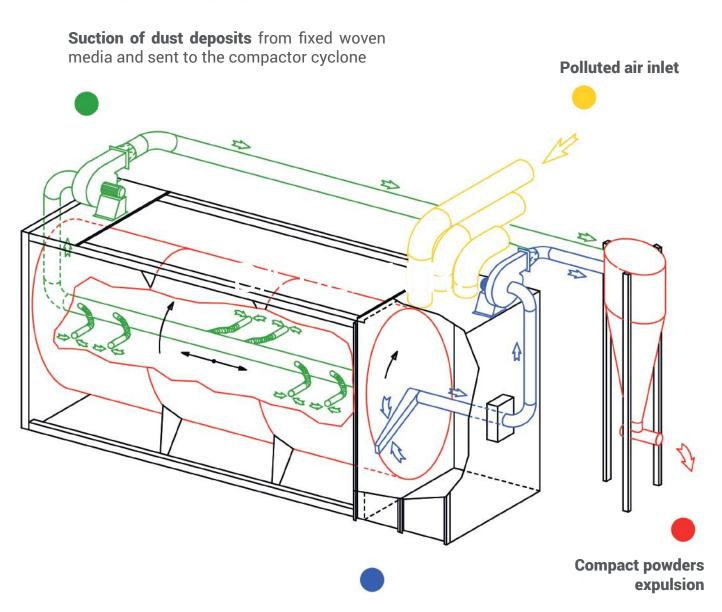
Suction of dust deposits on nylon net and sending the compactor cyclone
