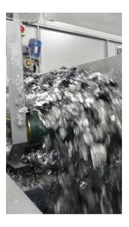
Traditional system provided a premelting of the shredded product in order to store it in vertical silos. Our application instead allows to avoid this step of heating and fusion because our storage boxes allow to standardize the product, store it and take it automatically with a dosing system that blends different types of products in order to send them to the extrusion line.
