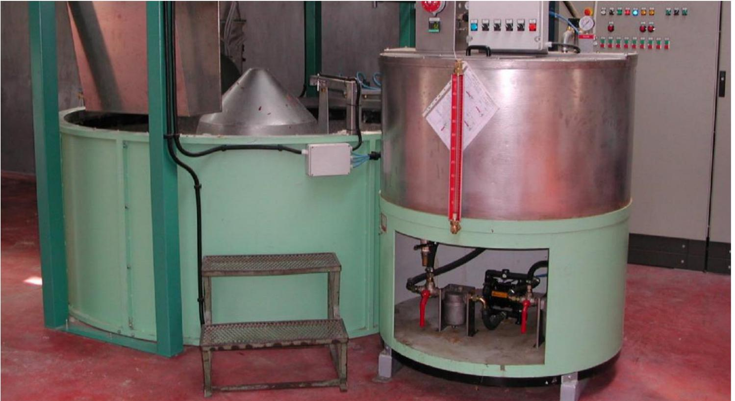
New studies and experiments carried out in view of the various problems connected with the application of oil and other additives have led to the realisation of the **new spraying system for direct application to the fibres being fed into the blending bins via conveyor belts.**
