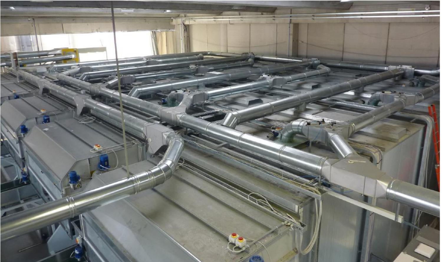
Setting system is very performing and allows to feed an extrusion line with more than **2.000 Kg/h** of regenerate products. Is handled automatically leaving to the operator the task to put the raw material on the conveyor stacker, from where the cycle do not need any manual intervention up to the storage of pallets of finished cips.
