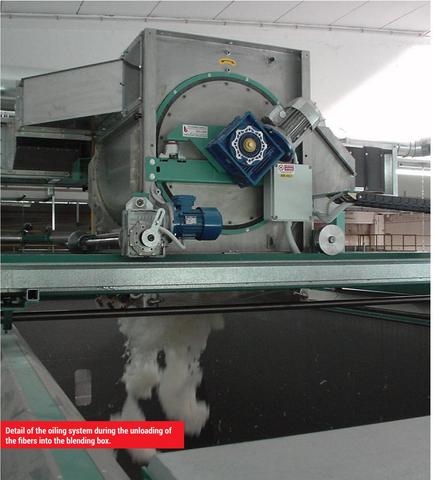
**Detail of the oiling system during the unloading of the fibers into the blending box.**
