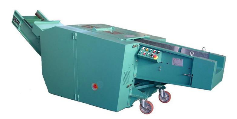
The rotating blades are helicoidally shaped which ensures a perfect cut on the entire 500 mm width and also distributes the cutting load over the length of the blades.
