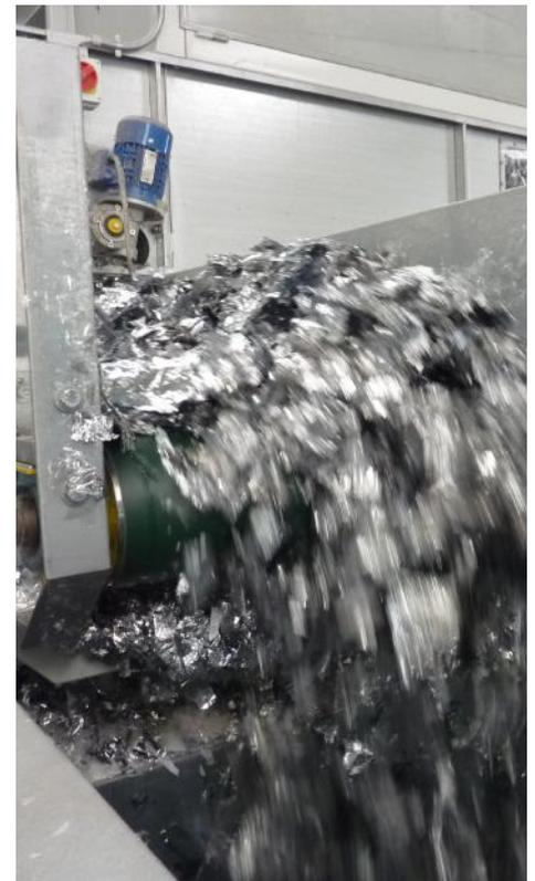
Traditional system provided a premelting of the shredded product in order to store it in vertical silos. Our application instead allows to avoid this step of heating and fusion because our storage boxes allow to standardize the product, store it and take it automatically with a dosing system that blends different types of products in order to send them to the extrusion line.
