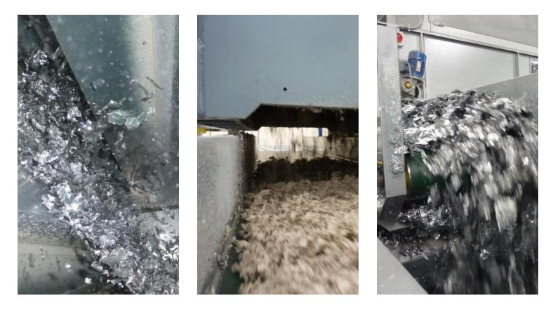
Traditional system provided a premelting of the shredded product in order to store it in vertical silos. Our application instead allows to avoid this step of heating and fusion because our storage boxes allow to standardize the product, store it and take it automatically with a dosing system that blends different types of products in order to send them to the extrusion line.
